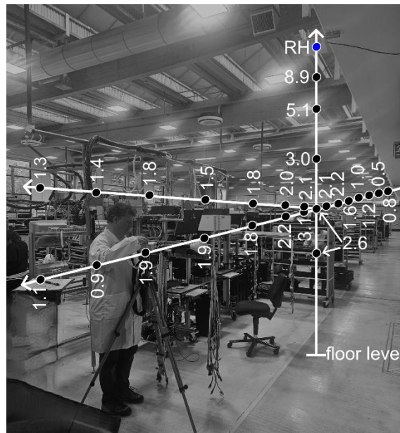
Figure 15: Extrapolated values of the measured electric field in the vicinity of a low-height pRRH in V/m. Measurements were taken at a height of 1.5 m in three directions at horizontal distances of 0.2, 0.5, 1, 2, 3, 4 and 5 m from the pRRH and directly below the pRRH at heights of 1, 1.5, 2, 2.5 and 2.8 m.
