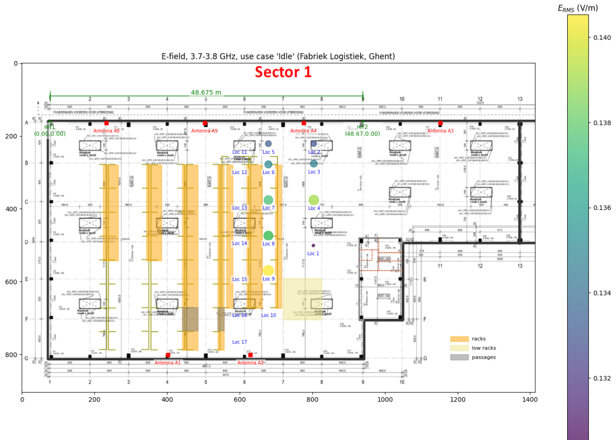
Figure 36: Measured averaged RMS E-field between 3700 MHz and 3800 MHz for the "Idle" (background) scenario in the pallet warehouse plotted on the ground plan of the pallet warehouse. The locations of the access points are indicated by the label "Loc" followed by a number. The RMS E-field values are represented as circles with color and radius scaled according to the field value.
