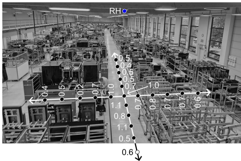
Figure 18: Results for detailed measurements under the pRRH mounted at the height of 5.9 m (located in the center). Measurements were done at the height of 1.5 m.
